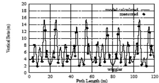
Figure 2: Measured and model calculated vertical betatron function with wiggler gap closed to 23.2 mm. The wiggler center is at 80 m from the injection point.
