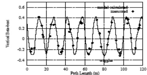
Figure 3: The measured and model calculated beta-beat between no wiggler and with wiggler gap 23.2 mm.
