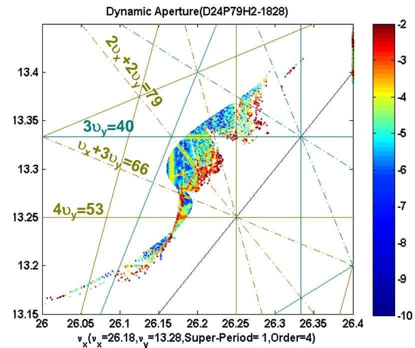
Tune diffusion rate  $D = \log_{10}((\Delta v_x)^2 + (\Delta v_y)^2)^{1/2}$  for tune difference
