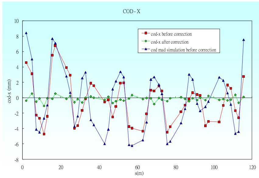
COD before correction (compared with model simulation with errors input) in SRRC Storage ring at commissioning stage in 1993. Corrected COD is shown too.
