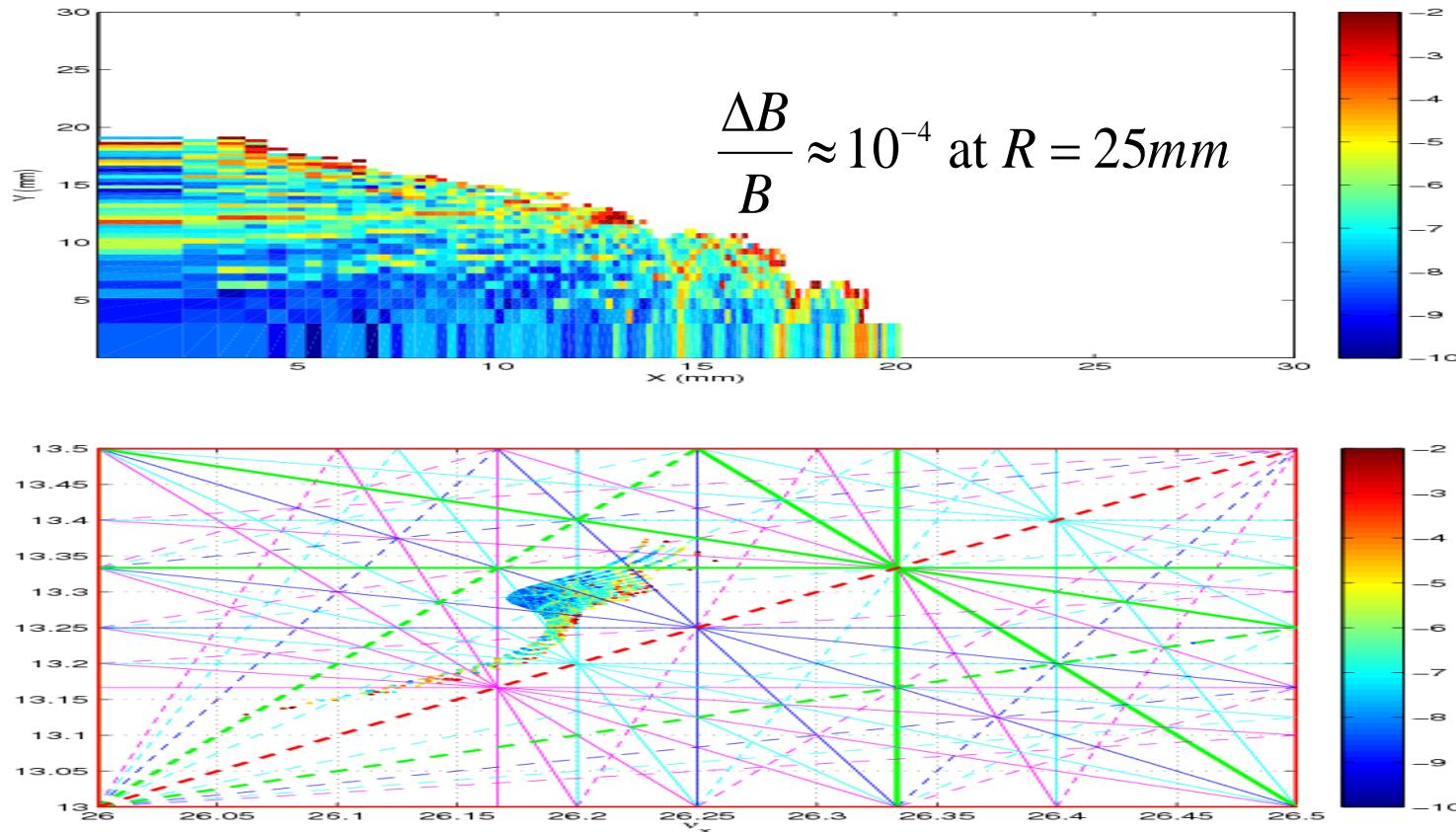
Tune diffusion rate  $D = \log_{10}((\Delta v_x)^2 + (\Delta v_y)^2)^{1/2}$  for tune difference
