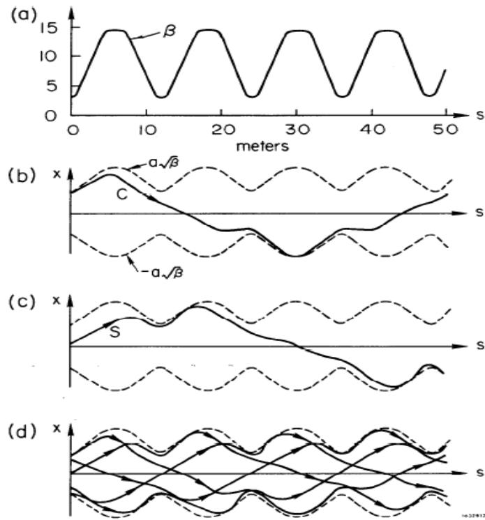
FIG. 12--(a) Betatron function. (b) Cosine-like trajectory for  $s=0$ . (c) Sine-like trajectory for  $s=0$ . (d) One trajectory on several successive revolutions.
