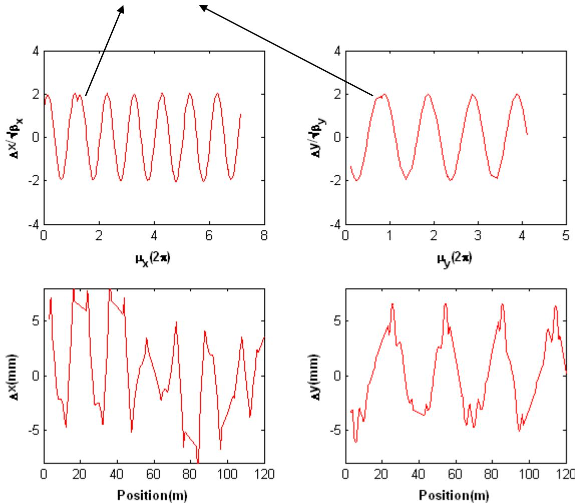
**Orbit distortions due to single dipole error kick in x and y planes in TLS ring, working point (7.18, 4.13) without errors.**
